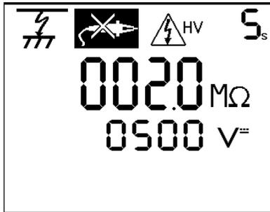
If an external connection e.g. a probe is required, the display will flash the connection icon. The user needs to connect the probe. The test can then proceed when the GREEN BUTTON button is pressed. At the end of each test in the test sequence, the display will indicate the result.
